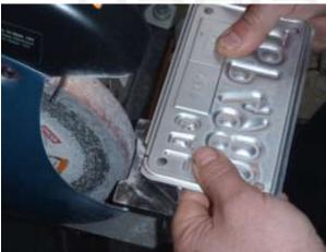
Use a grinder or Dremal to notch plate frame
